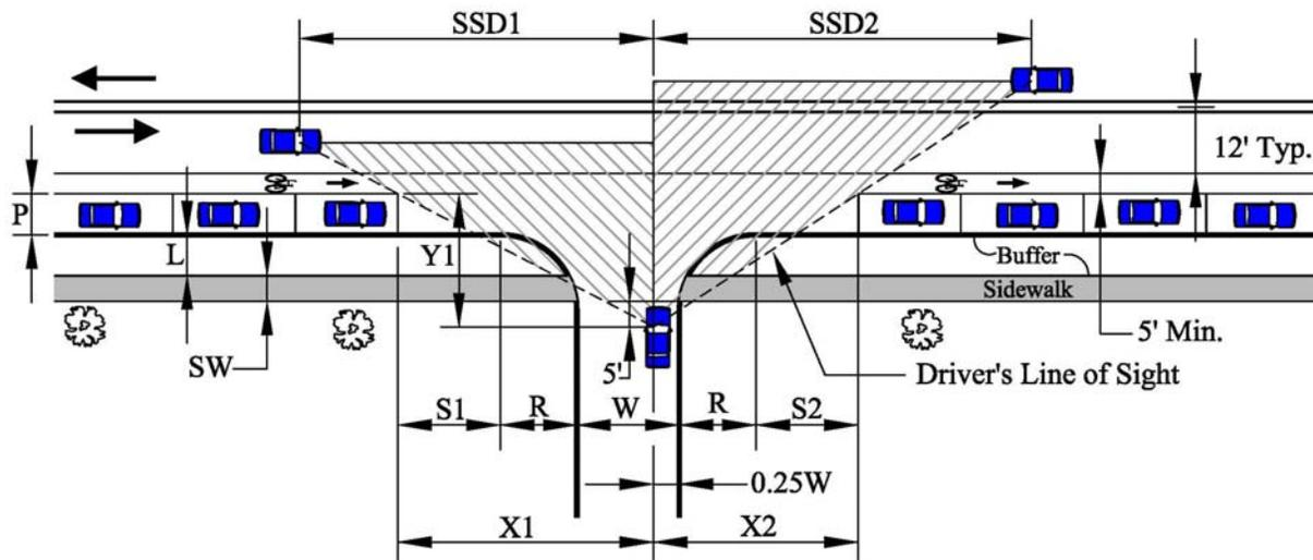
**Figure 3. Components of On-Street Parking with a Buffer Strip**
