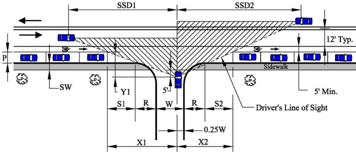
**Figure 8. Components of On-Street Parking without a Buffer Strip**
